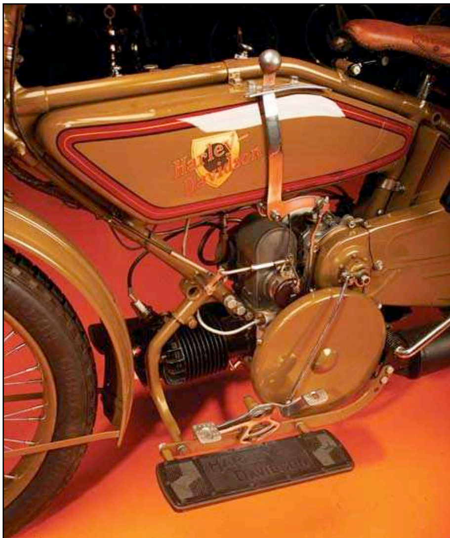
The clutch is operated by the rider's left foot.
