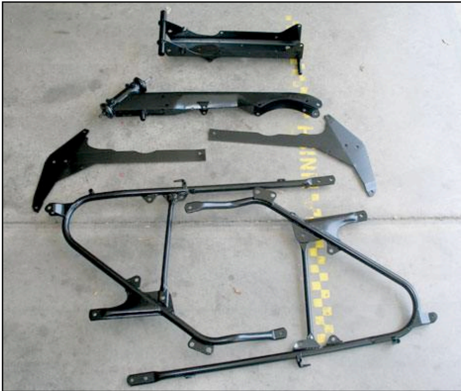
The frame is assembled from six different parts. From top, the central spine, front with steering head, two reinforcement plates, and the left and right sides.
