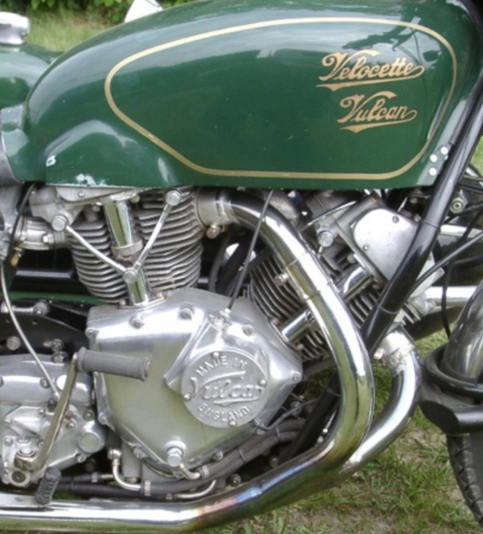
Velocette Vulcan. 1000cc. A one-off built by the owner, Bob Higgs; mating two Velocette 500cc barrels in "V" configuration.
