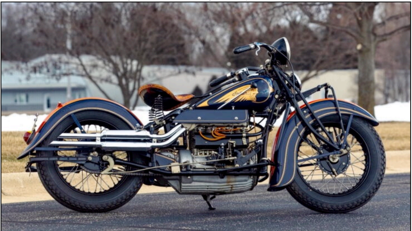
The inline-four cylinder engine was mounted longitudinally, so it was quite narrow in the frame
