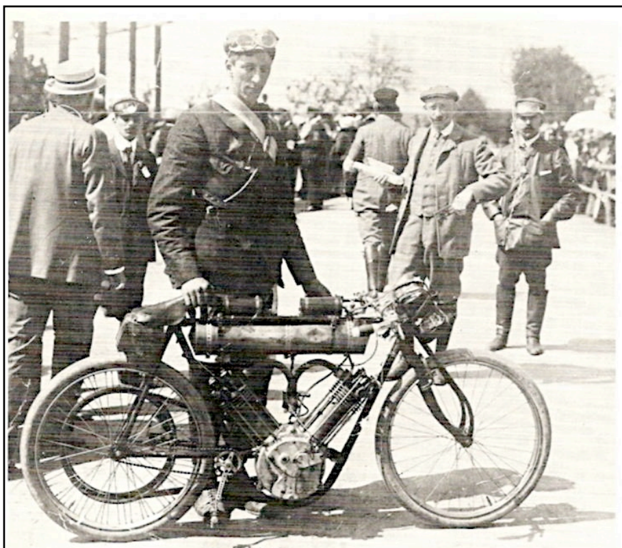
C. B. Franklin with the racing model on which he represented England in the Austrian International Cup Race of 1906. The engine is a specially-prepared 8hp 90° vee-twin racing engine with bore and stroke dimensions of 85 x 85mm. (Photo: Haringey Public Libraries)
