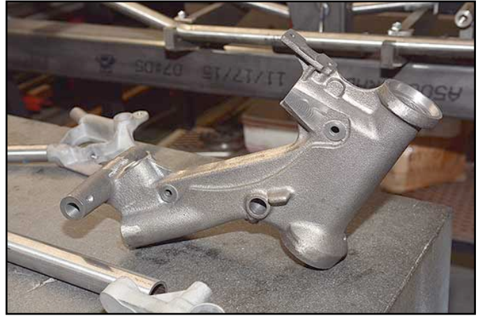
Engines coming together at Kiwi Indian and a new cast head stock (shown) ready to become part of a Chieftain frame.
