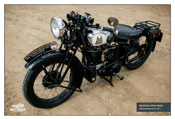
motorcycle, making it quite cumbersome. The V-shaped four-cylinder engine was a solution to this problem. Thanks to the power of the four cylinders and the compactness of the motor, the Matchless Silver Hawk had a sporty look, which was exactly what Collier had in mind. Another advantage of this model was the soft rear suspension.
