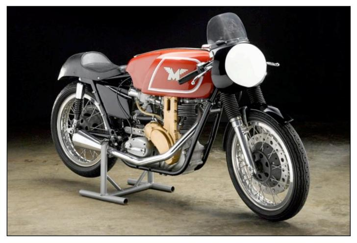
With a kerb weight of ~150 kilograms and a little over 50 bhp, the G50 provided stiff competition for the likes of the Norton Manx – although the Norton was more powerful, it was also heavier, so the Matchless could make up time in the corners.
