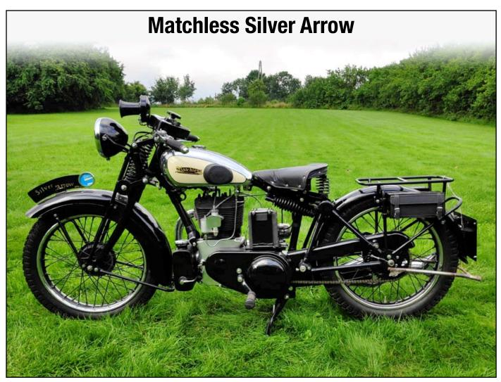
Matchless Silver Arrow motorcycle, years of production: 1929-1933.V-twin engine 397cc (24ci), power 16HP at 5000rpm, weight 140kg, top speed 105 km/h (65mph). Of the 1700 odd machines produced only about 40 are known to have survived.
