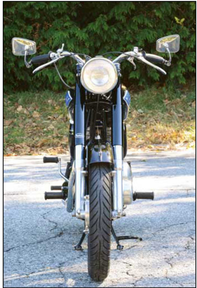
Straight-on shot shows how slender the Model 16 is. Tires are modern Avon Roadriders.
