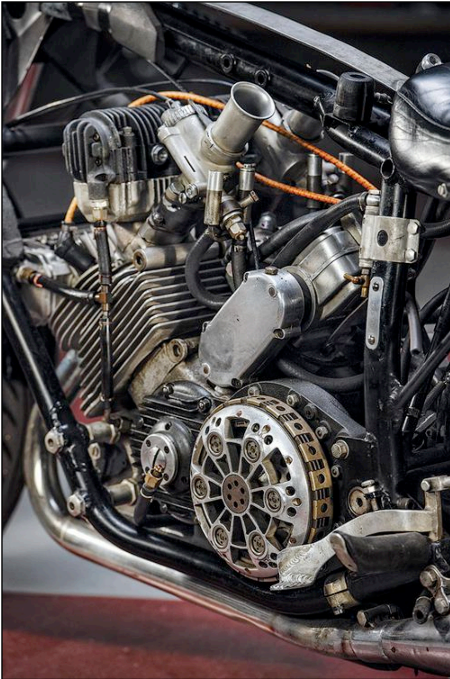
Dry clutch, unitized engine/gearbox and gear primary drive made the AJS advanced for its day.
