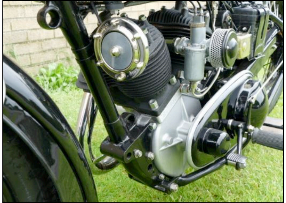
A view of the AJS Model 37/2 990cc V-twin engine. Photo credit: Spicer Auctions
