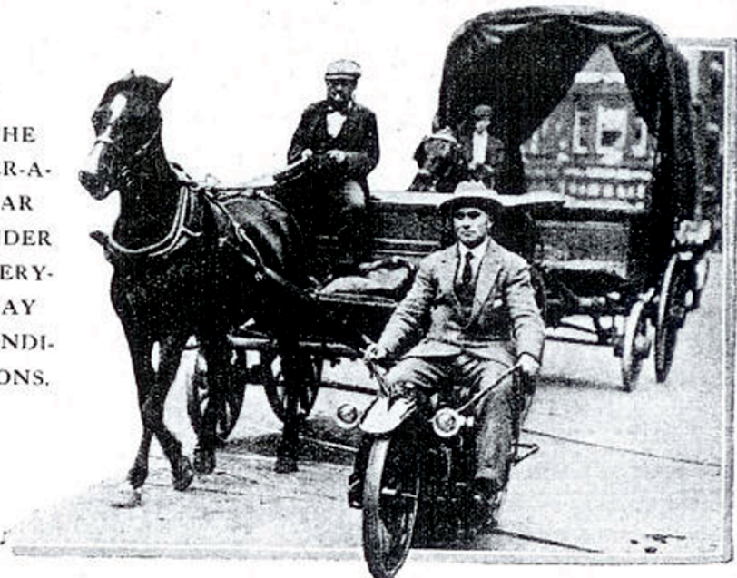
The low centre of gravity makes the Ner-a-Car delightfully easy to control in traffic.
