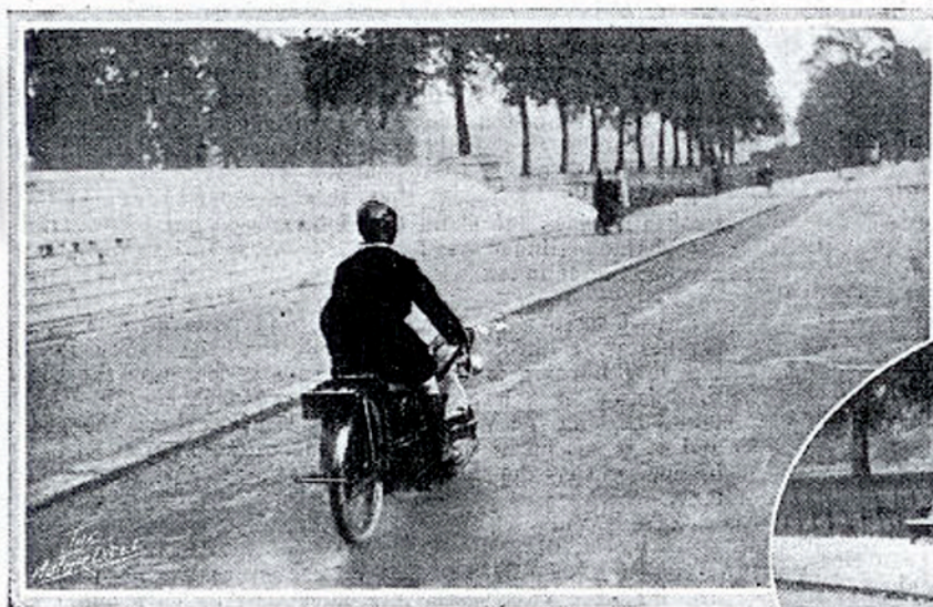
Nearly all the weight of the Ner-a-car being carried below the level of the hubs, there is little tendency to skid. The riding position is comfortable, and, taken all round, the machine is very controllable.
