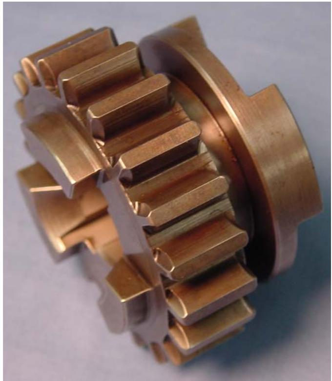
Limited number of newly manufactured second gear pair for the vintage o.h.v. Douglas motorcycle three-speed gearbox. On offer are the 19-tooth mainshaft slider gear and its mating 18-tooth layshaft gear.
